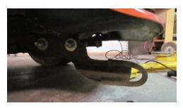
Alternatively, bolt on a tow arm using the same mounts. Note the arm clears the dam and presents a angle iron 'L' at about bumper level.
